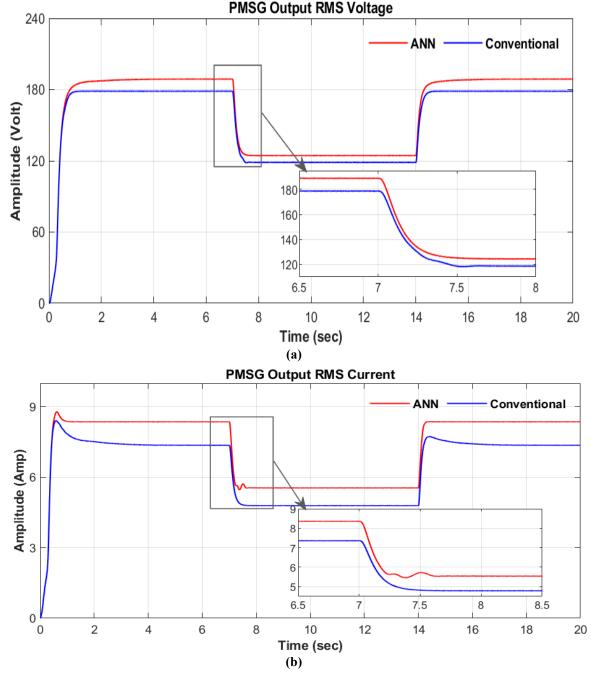
Fig. 4.2 Comparative Simulation Results of ANN and P&O MPPT Algorithm during Step Change in Wind Speed from 12-8-12m/s, Waveform of PMSG (a) RMS Voltage (b) RMS Current
