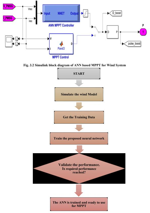
Fig. 3.3 Flow chart for Training Procedure of ANN based MPPT for Wind System
