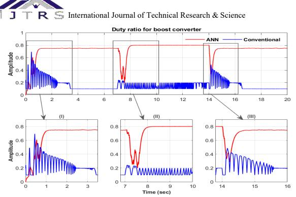
Fig. 4.3 Comparative Simulation Results of ANN and P&O MPPT Algorithm during Step Change in Wind Speed from 12-8-12m/s, Waveform of Boost Converter Duty Ratio
