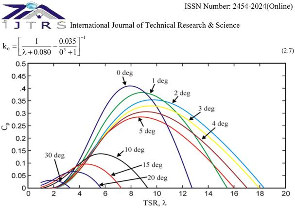
Fig. 2.1 C<sub>p</sub>-λ Characteristics at Different Pitch Angles (θ)
