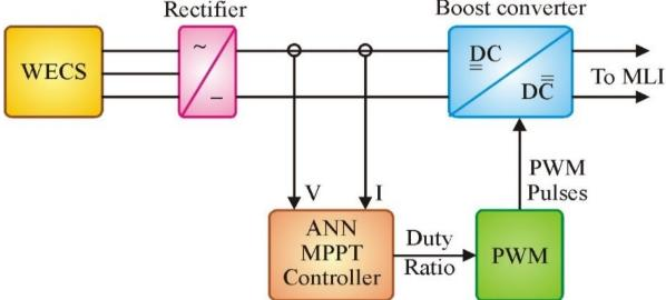
Fig. 3.1 Block Diagram of ANN MPPT Controller
